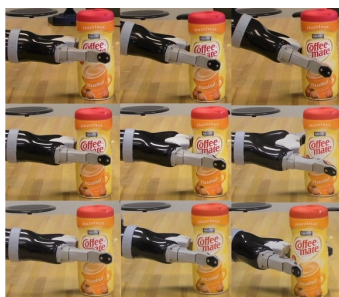
Fig. 8. Visualization of \delta R (top row), \delta P (middle row) and \delta Y (bottom row) for 0^\circ , 10^\circ and 20^\circ (left to right).
