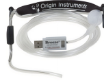
Fig. 2. Top: Study setup. Participants use a sip/puff interface to teleoperate a robotic arm to retrieve a cup from a shelf and place it on the table. Bottom: The sip/puff interface.
